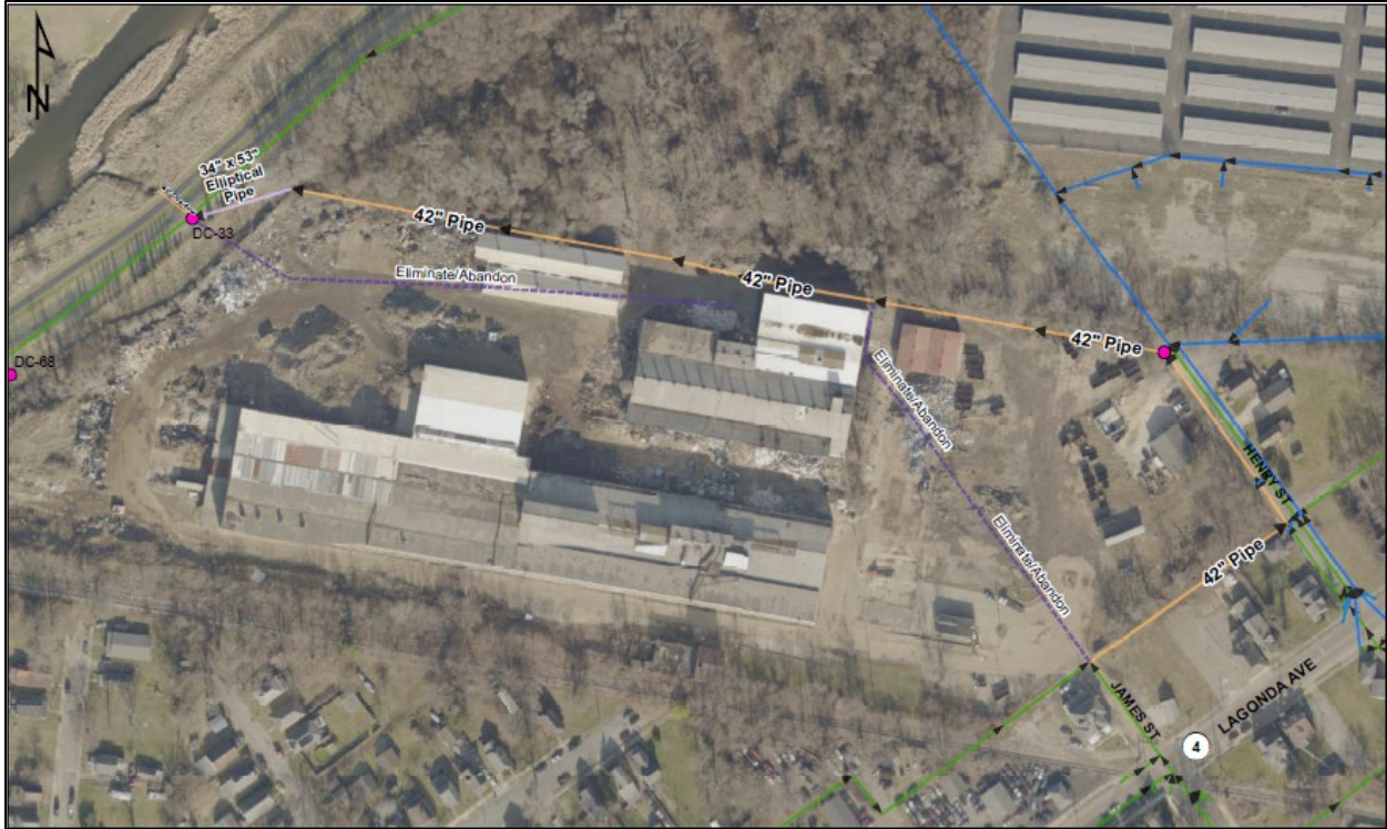
Figure 2. Map of the project area. The orange line represents the new sewer line
