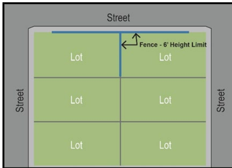
Figure 1120.04.1: 6-Foot Fence Height Limit
