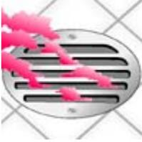
Cover floor drain with fine screen and empty into garbage can as needed.
